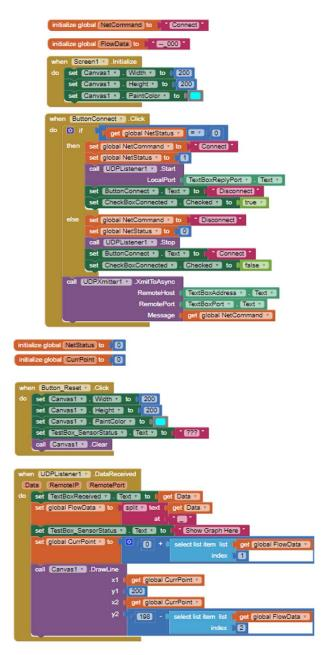
Fig. 7. The main parts of the IoT monitoring application for smart phones, as implemented using the MIT App Inventor visual programming environment
