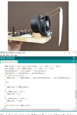
Fig. 4. Experimental controllable air flow unit utilizing the distance from a piece of paper in front of the fan as feedback parameter (top part) and an indicative implementation using the Arduino IDE (bottom part)
