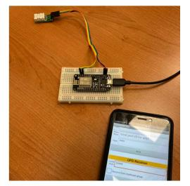
Fig. 6. Experimental IoT system for wireless monitoring of air temperature and humidity, via a smart phone
