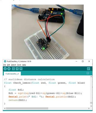
Fig. 5. An RGB color sensor as the key component for classifying objects, such as leafs or fruits, (top part) and the corresponding code part calculating the Euclidean distance metric (bottom part)
